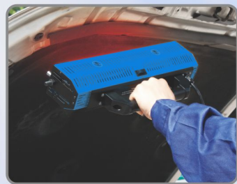
Drying in hard reach area or small area
