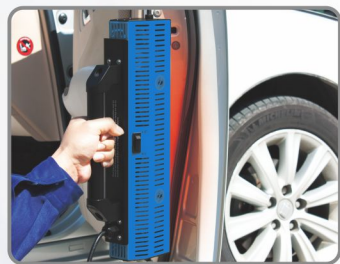
Softening trim moulding
