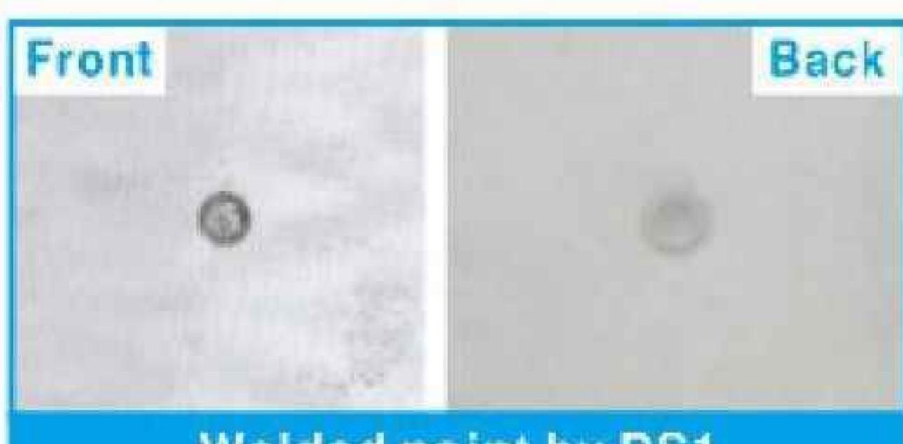
Welded point by DS1
