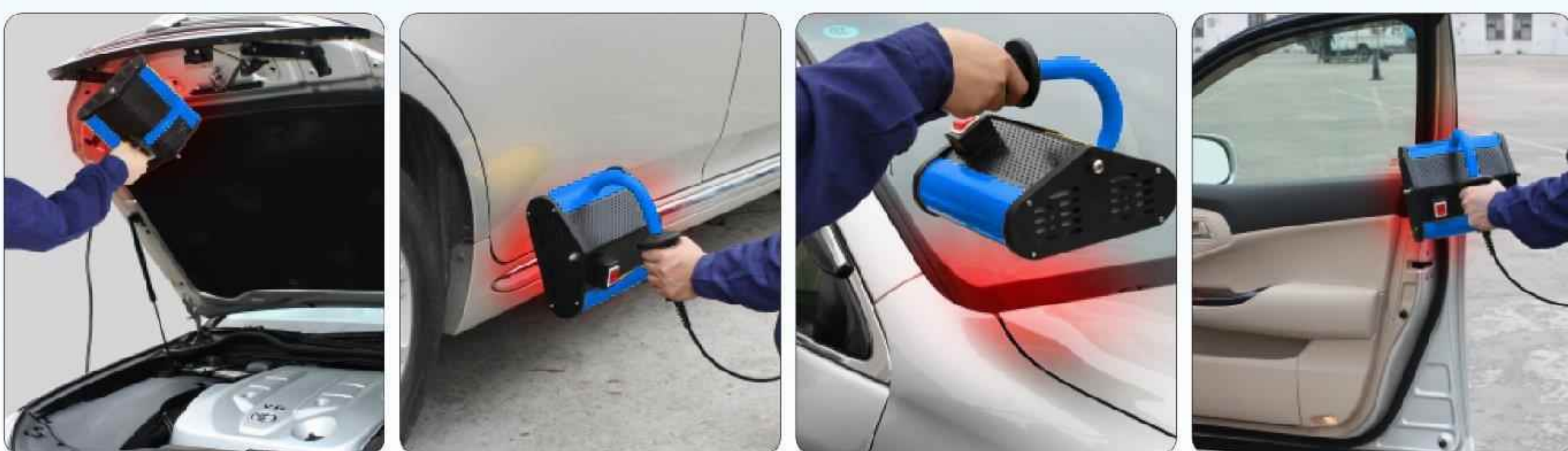
Drying in hard reach area or small area Removing strip Replacing windshield Soften trim moulding
